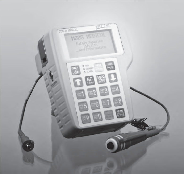
Figure 5-36 ■ Ambulatory pump: 6000CMS Ambulatory electronic infusion device. Capable of infusion modes including continuous infusion, patient-controlled analgesia, patient-controlled epidural analgesia, subcutaneous infusion, total parenteral nutrition, and intermittent infusions. (Courtesy of Moog Medical Devices Group, Salt Lake City, UT.)
